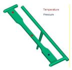
Figure 1: Tensile bar geometry with the locations of the pressure and temperature sensors
